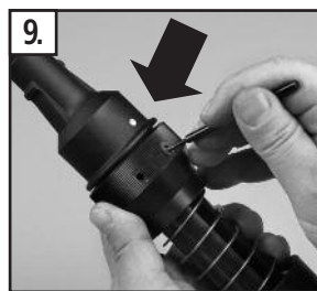
Push in green pin and rotate until red dot is shown
