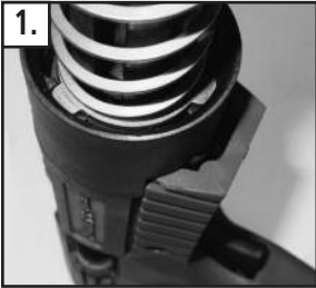
1. Turn piston return spring out of engagement slots on piston return spring sleeve
