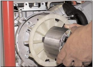
Step 4 - Install rotor thru bolt (install short threaded end of rotor thru bolt in engine shaft until threads run out), washer and nut, using a ½ socket. Torqued at 120-144 in lbs
