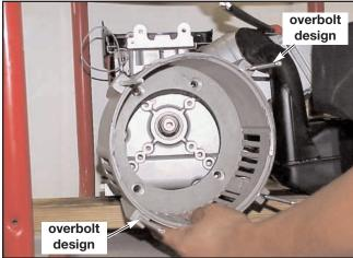
Step 2 - Install washer, lock washer and bolt using a 9/16 socket. The four bolts generators will be torqued at 204-264 in lbs.
