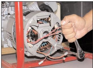
Step 7 - Remove one isolator and washer and bolt from the old style bearing support. Install the washer and isolator in the center of new style bearing support. Remove the 2x4, which was supporting the gen head, Line up the isolator with the hole in the frame which best centers the gen head and bolt the isolator to the frame. Torqued at 96-120 in lbs.
