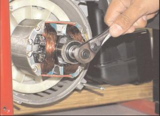
Step 5 - Install stator
