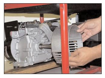
B- Installation of the new style Gen-Head For 2500kw - 3500kw generators
