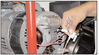
Step 9 - The ground lug will need to bolted to a hole on the support bar to the right of the gen head. Torqued at 90-120 in lbs.
