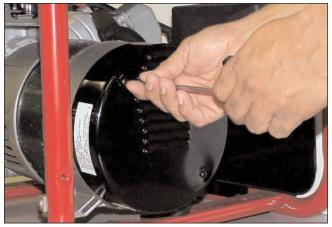
**Step 2** - Once the end cover is removed, disconnect the wires to the capacitor and the Stator.
