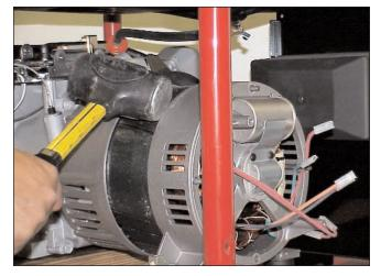
**Step 5** - Remove the stator.
