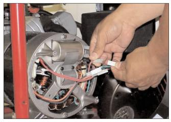
**Step 3** - Remove the grounding lug and the nuts from the isolators underneath the support bar on the frame.
