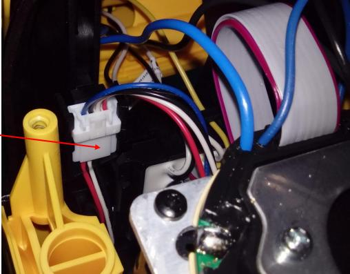
Unplug the 4P male connector from the speed dial wire harness and plug the service wire harness into it. Power the unit up with a battery and press the switch trigger.
