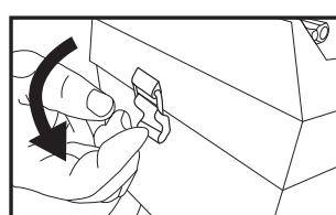
**4** Connect engine start connector to the battery box
