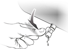
Drain valve (open)
