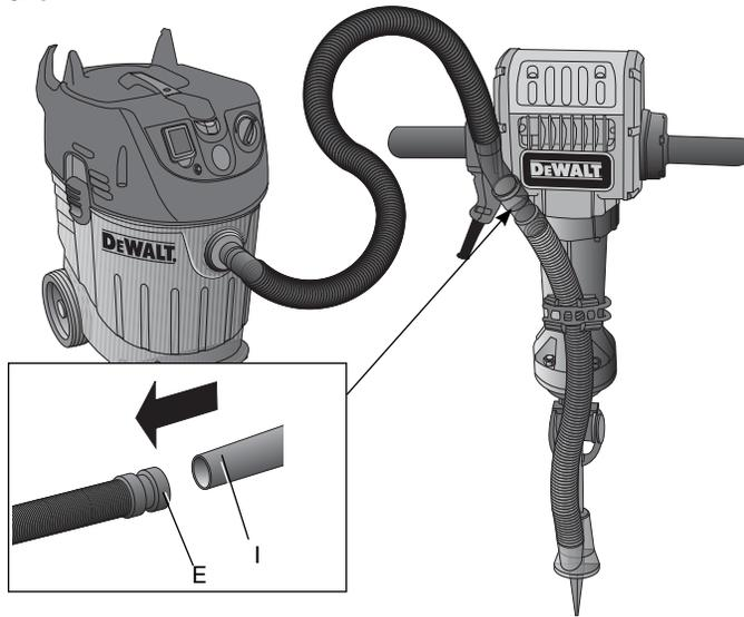
Push dust extractor vacuum hose nozzle (I) into connection point (E) until tight. For a more secure connection use the AirLock connection system.
