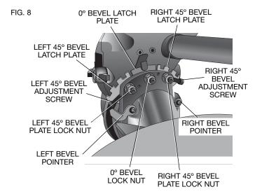
45° bevel - Left Result Width 12.9" (328 mm) Max. Height 2.4" (61 mm)
