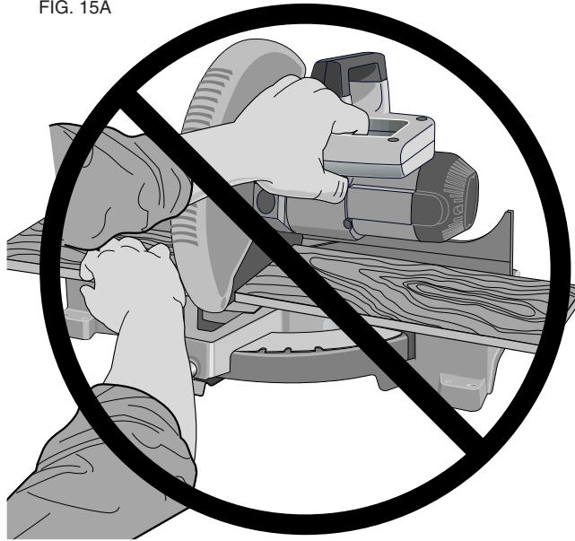
IMPROPER HAND POSITION
