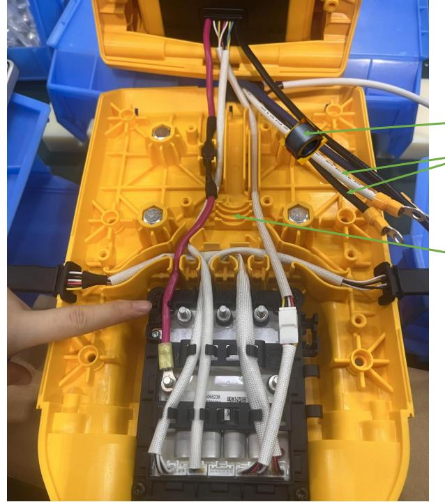
Add Ferrit core around UVW – put each cable separately through the core
