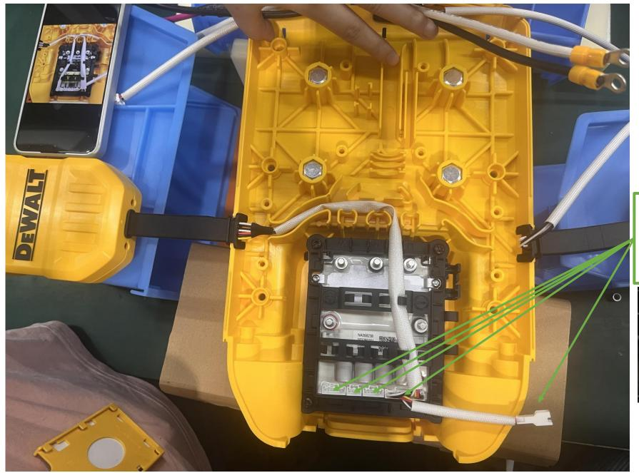
Add Silicone Grease NA218891 to all wire-to-wire headers BEFORE connecting. Fill up header. Also on BLEM module before connecting!
