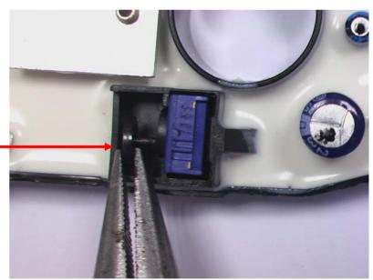
WITH BUTTON BACK IN PLACE DEPRESS THE BUTTON AND YOU SHOULD HEAR THE SWITCH CLICK ON AND OFF
