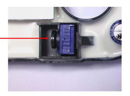
IF THIS BUTTON IS MISSING THE TRIGGER ON THE NAILER CANNOT WORK AND THESE MODULES ARE USELESS
