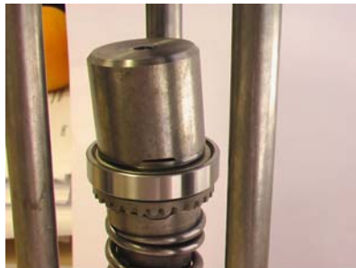
COVER TOOLING INCORRECTLY SEATED
