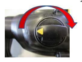
PLACE UNIT IN HAMMER DRILL POSITION AND TURN THE MODE SELECTOR CLOCKWISE 180 DEGREES TO THE SERVICE POSITION
