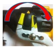
WHEN IN THE DRILL POSITION THERE WILL BE SOME RESISTANCE AND THE USE OF SOFT GRIP WRENCH MAY BE NEEDED – (use soft grip wrench to avoid damage to the mode selector)
