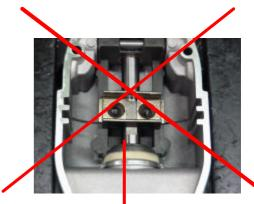
Yoke is screwed down with flats showing which will cause failure of shaft rotating causing blade alignment to be out or sticking shaft
