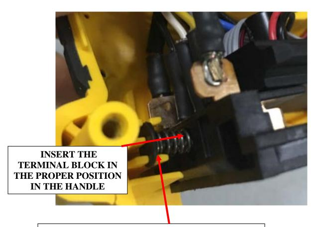
INSERT SPRING INTO RECTANGULAR POCKET OF THE TERMINAL, WHILE PUTTING SUPPORT INTO THE NEST IN THE HANDLE
