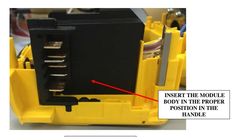
\* ENSURE TERMINAL BLOCK AND MODULE ARE FULLY SEATED ENSURE EVERYTHING IS PROPERLY SEATED IN ITS PLACE PRIOR TO PLACING THE COVER ONTO THE ASSEMBLY
