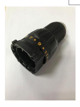
REMOVE GEARCASE AND CHUCK AS ABOVE
