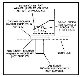
Stationary air compressors must be bolted to the floor. Bolting holes are provided in the base feet. Mount the air compressor on a solid, level foundation. Support compressor weight evenly on all four feet. Solid shims may be used if necessary.
