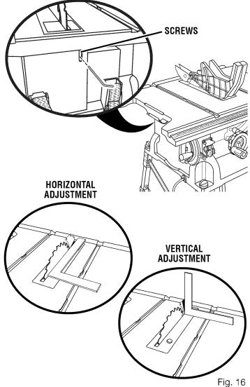
If the riving knife is out of alignment with the saw blade, adjustment is needed. The riving knife must be in alignment front to back (horizontally) and top to bottom (vertically).
