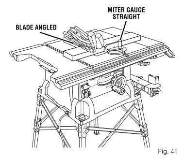
NOTE: The hand closest to the blade should be placed on the miter gauge lock knob and the hand farthest from the blade should be placed on the workpiece.
