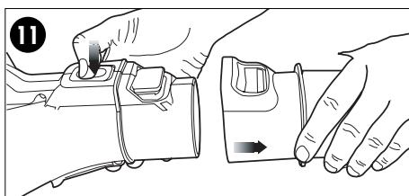
**REMOVING BLOW TUBE, VAC TUBE OR COLLECTION BAG (FIGURE 11)**
