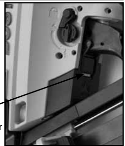
Dial-A-Depth® Fastener Control Adjustment
