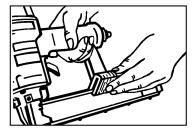
Use stick of staples to move cover spring to one side and drop over core of magazine.
