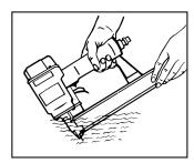
Tar and dirt may build up on the nose and contact arm. This can prevent correct operation. Remove any buildup with kerosene, #2 fuel oil or diesel fuel. Do not immerse the stapler into these solvents beyond the bottom of the frame to avoid getting the solvent into the drive cylinder.
