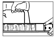
3. Depress pusher latch pin with thumb and allow pusher to slide forward to engage staples. On narrow crown models pull pusher back out of notch and allow to slide forward.
