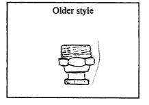
On these older style units, the drain valve was located in the center bottom of the tank, and had very large threads. This part is no longer available. Refer calls to Service Centers.
