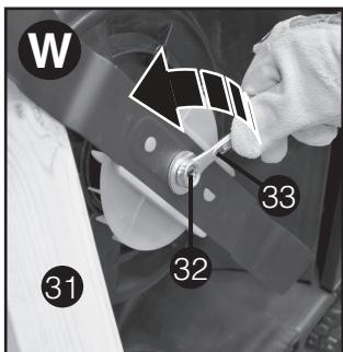
4. Remove bolt and washer (34). Pull off blade (35) as shown in **Figure X.** The fan (36) should not be removed. Examine all pieces for damage and replace if necessary.
