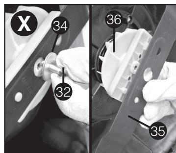
5. The blade can only be attached to the fan in one direction. To reassemble, line up the D-shaped hole of the blade with the D-shaped post of the fan, ensuring the writing on the blade faces out away from the mower.
