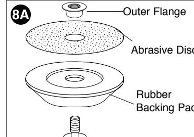
3. Tighten the abrasive disc as shown in Figure 9 by depressing the spindle lock button and turning the abrasive disc by hand.
