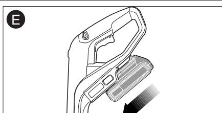
8) **Depress the lock off button** (as shown here) in either direction and simultaneously pull the trigger. You do not need to continue to depress the lock off button during operation.
