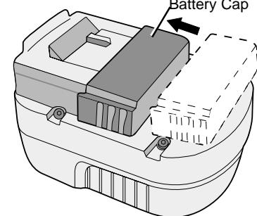
⚠ **WARNING!** Do not store or carry battery so that metal objects can contact exposed battery terminals. For example, do not place battery in aprons, pockets, tool boxes, product kit boxes, drawers, etc. with loose nails, screws, keys, etc. without battery cap. Without cap in place, battery could short circuit causing fire or burns or damage to battery.
