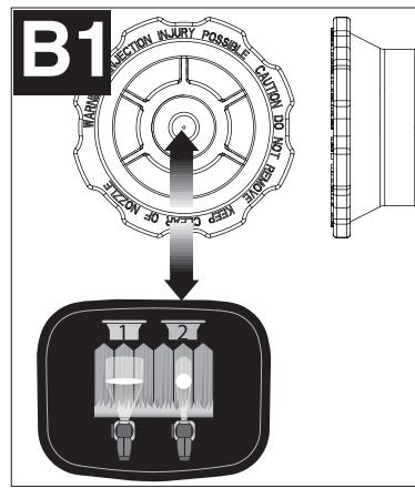
**Cone nozzle (blue - figure B1)** - The cone nozzle spray pattern is more concentrated. Use this nozzle for items that are too small for the fan nozzle. This is the spray nozzle that is identified as number 2 in the diagram on top of the sprayer.
