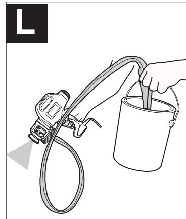
3. Aim the sprayer at a piece of scrap wood or cardboard. Squeeze the trigger and hold until all air is out of the system and material is flowing freely out of the sprayer tip. This could take up to three minutes.
