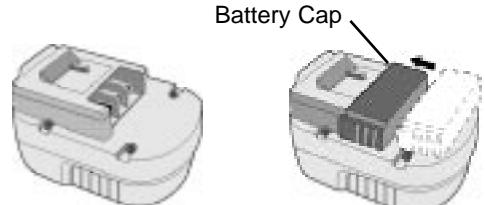
**⚠ WARNING!** Do not store or carry battery so that metal objects can contact exposed battery terminals. For example, do not place battery in aprons, pockets, tool boxes, product kit boxes, drawers, etc. with loose nails, screws, keys, etc. without battery cap. Without cap in place, battery could short circuit causing fire or burns or damage to battery.
